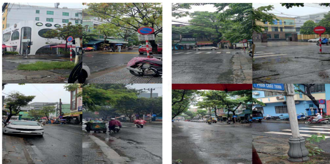
■ Fig. 1. Examples of Mosaic augmentation applied to traffic sign images
